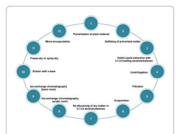
**Figure 1:** Bioprocess for the production of glucosinolate-based dietary supplement [47].
