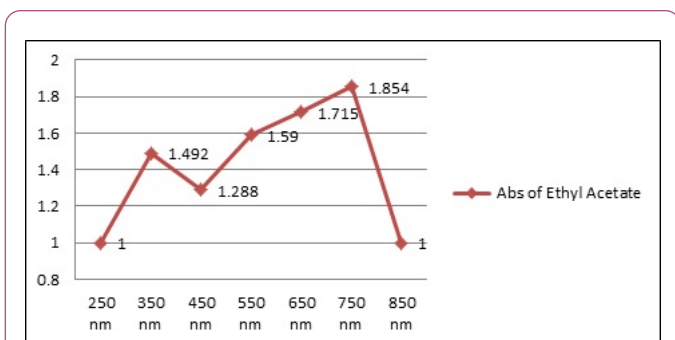
Figure 1: Absorbance of Ethyl acetate with the oil-rich extract obtained from kale leaves using UV vis Spectrophotometer.
