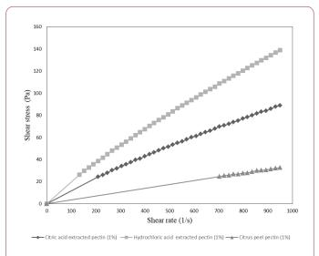
**Figure 3:** Flow behavior of the pectin extracted using hydrochloric acid or citric acid and a citrus peel pectin at 1% concentration.
