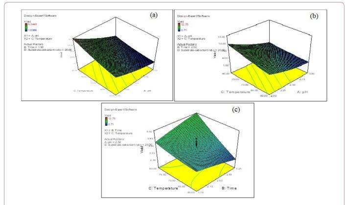
**Figure 1:** 3D surface plots for the yield of pectin extracted from watermelon rind using hydrochloric acid. A): Effect of pH and temperature; B): Effect of pH and temperature; C): Effect of time (h) and temperature.
